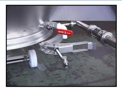
Very big opening, conical butt type. Very easy opening. The cake is collected on a suitable trolley on wheels.
